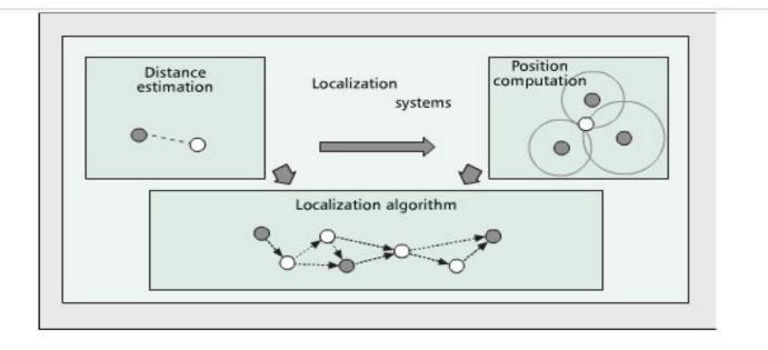
Distance/angle estimation: Estimating position related parameters between two nodes.
